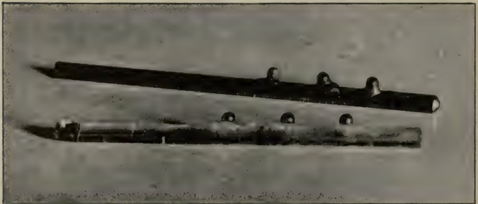
FIG. 56. The metal balls are fastened to the iron and glass rods with drops of wax.
